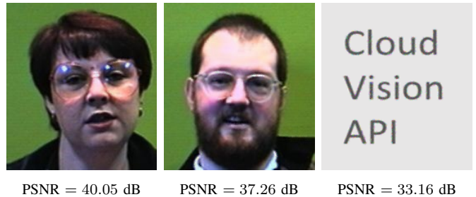
Fig. 6: The restored images, generated by applying the weighted-average filter [24] on the noisy images of figures 3 and 4. Captions show the PSNR values with respect to the original images. Although the API fails to detect the face in the noisy face images, it correctly detects the same face attributes for restored images as the original images. Also, unlike the noisy version of the text image, the API correctly reads the text within the restored image.
